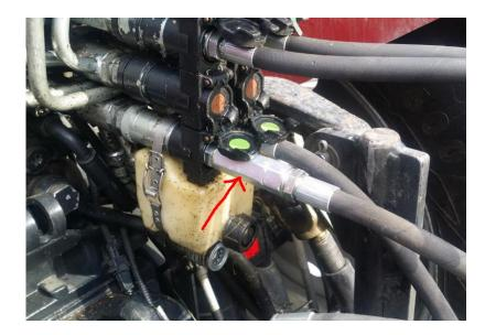
Release the quick coupling from the non-return valve to relieve the oil pressure between them. Screw parts together and try again. If possible, this hose can be routed in a free return section to avoid pressure on this side.
